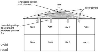
Figure 7: Fire that starts in roof void provides potential for downward fire spread
