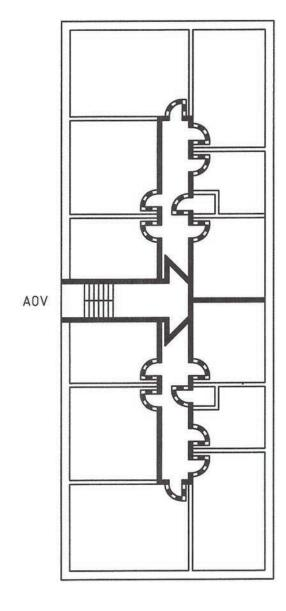
Figure 16b: Small building of not more than two dwellings per storey and protected internal entrance halls
