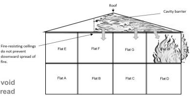
Figure 8: Fire that spreads into roof void provides potential for downward fire spread
